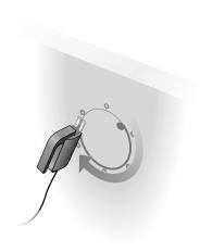
Use a half-round file or wood rasp to smooth out any roughness in the speaker hole you have cut.
