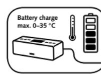
Charge the battery at an ambient temperature of 0–35°C
