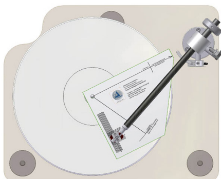
Pic. 10: Alignment of the cartridge
