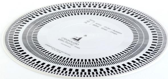
If you choose the side without the *Speed Light* source, you can use the regular light source for the installation, either 50 Hz (outer scales) or 60 Hz. The scales are graduated in three different reading options: 33,3 Hz, 45 Hz and 78 Hz (starting from the outer diameter).
