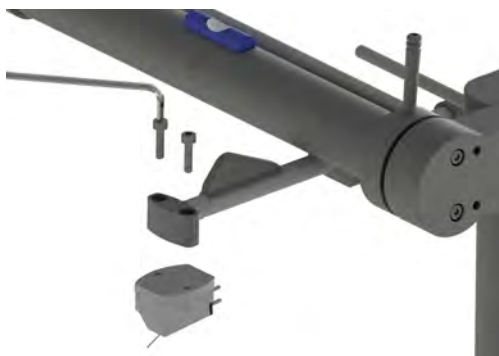
Pic. 6: Mounting the cartridge
