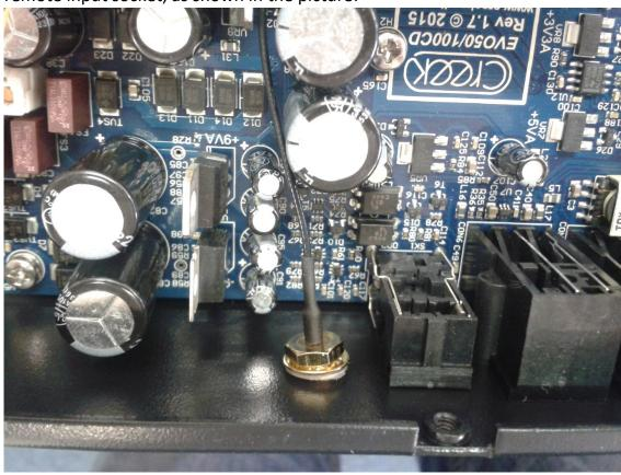
3. On the opposite side put the larger white insulating washer on the socket. Now fit the gold nut and screw it-up tightly, using pliers or a small spanner, like shown on the picture:
