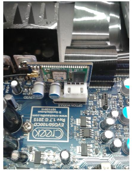
Make sure that pins on both sockets match each other and no pins are left unconnected.
