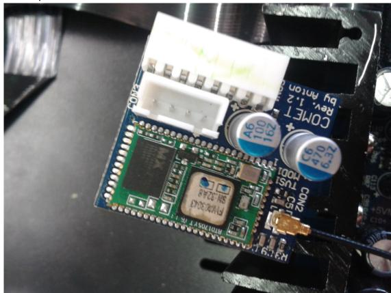
2. Plug the Comet BT PCB into the socket on PCB with capacitors pointing towards the back panel, like shown on the picture:
