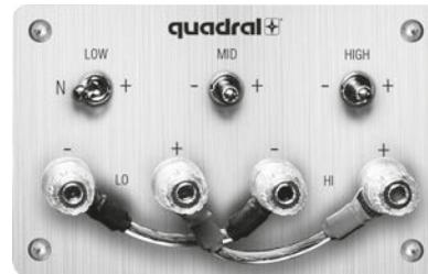
Make sure you use the correct polarities in these modes and that you remove the jumpers on the speaker terminal to avoid damaging your amplifier.
