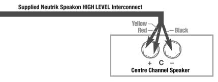
• If connecting a REL as a dedicated rear channel sub, connect the black wire of the REL to either the left rear or right rear negative speaker terminal; connect the yellow wire to the left rear positive speaker terminal; connect the red wire to the right rear positive speaker terminal. If the amplifier is of balanced differential design, please follow the instructions in the section above labeled Differential Connection.
