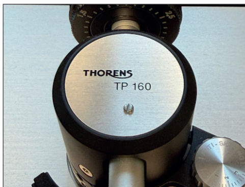
Fig. 8 Installed counterweight with scale for tracking force (value 2) and adjustment wheel for magnetic anti-skating.
