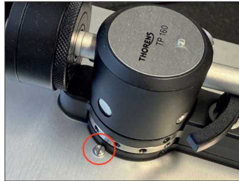
Fig. 24 Adjustment screw for the limit switch.
